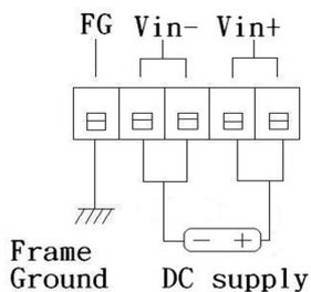
\*For 48VDC typical model(DIN-SW5G44x4)
