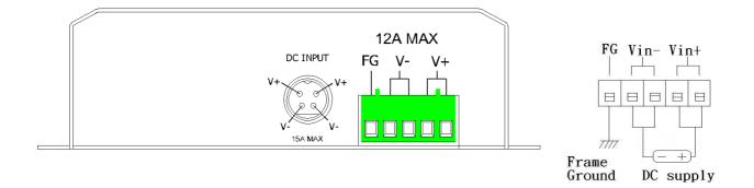
The DIN-4P connector on the rear panel can be also used for power input, you can use an AC/DC adapter with DIN-4P connector directly, recommend adaptor MS-180-56. (OPTION)
